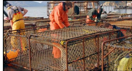
Rectangular crab traps Made from galvanized steel and are covered with polypropylene mesh Dimensions: 89" x 89" x 36"
