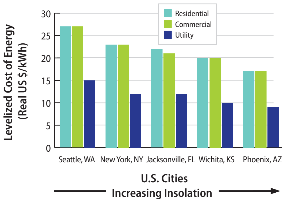
Figure 3.1 LCOE for residential, commercial, and utility-scale PV systems in several U.S. cities 21 (NREL 2011)
