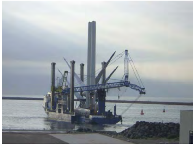
Figure 5.12. The Sea Energy Leaving Port with Two 55 m Towers, Two Bunny-Eared Nacelles and Two Additional Blades
