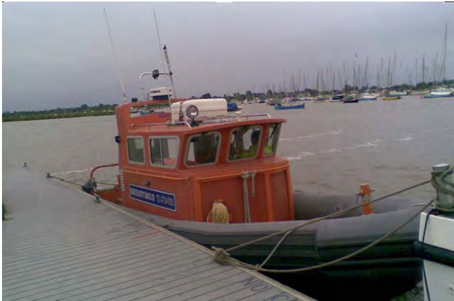
Figure 6.9. A Rigid Hull Inflatable Boat Used for Personnel Transfer and Utility Work at Gunfleet Sands
