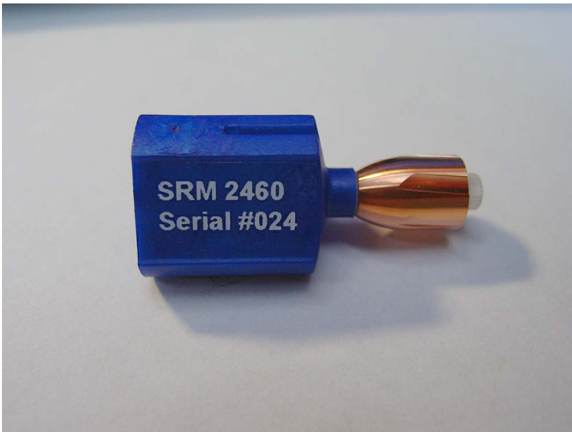
Figure 1. A NIST SRM 2460 standard bullet is mounted on a blue stub. One of the six highly uniform, land engraved areas (trapezoidal in shape) is clearly visible.
