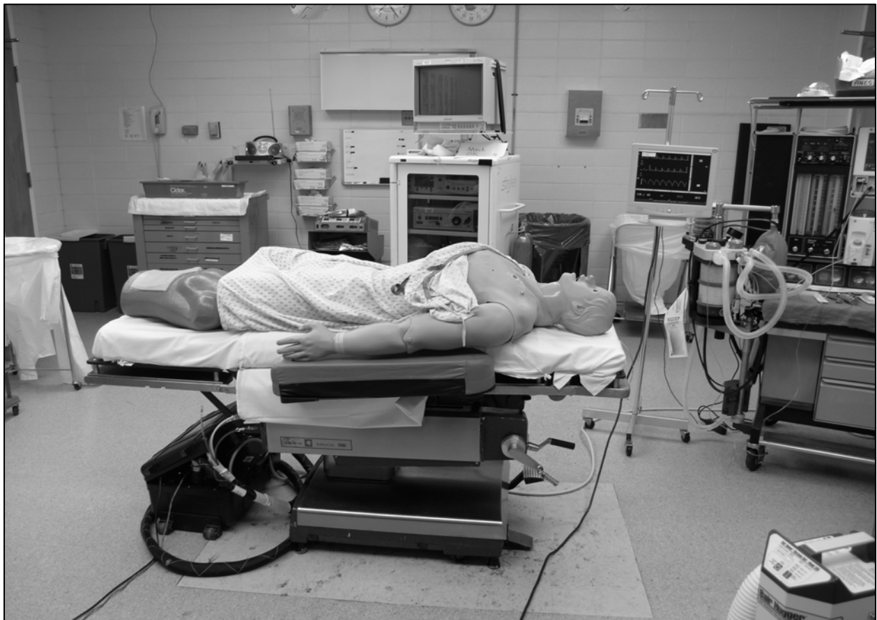
Figure 1. The two main components of the MMOR simulator equipment include a portable computerized mannequin combined with an inanimate cholecystectomy model. The mannequin rests on the OR table with the cholecystectomy model at the foot of the bed. The mannequin control box is placed underneath the OR table and is connected to the computer via an Ethernet cable (lower left) and an air compressor via tubing (middle right).
