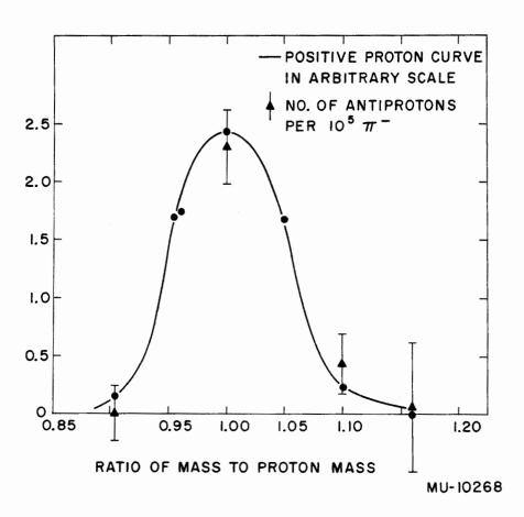
Fig. 4. The solid curve represents the mass resolution of the apparatus as obtained with protons. Also shown are the experimental points obtained with antiprotons.
