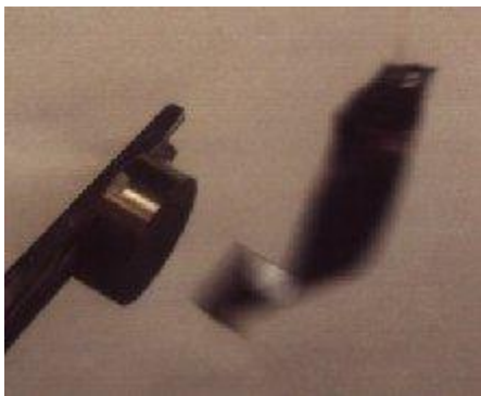
Photograph of a coating of the V[TCNE] x magnet on a Teflon tape being attracted to a Co 5 Sm magnet at room temperature in the air.
