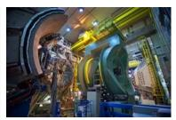
Photo courtesy of Brookhaven National Laborator The PHENIX detector at Brookhaven National Laboratory's Relativistic Heavy Ion Collider (RHIC) records many different particles emerging from RHIC collisions, including photons, electrons, muons, and quarkcontaining particles called hadrons. The detector is shown here in a disassembled condition during maintenance.
