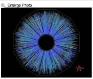
Image courtesy of Brookhaven National Laboratory End view of a collision of two 30-billion electron-volt gold beams in the STAR detector at the Relativistic Heavy Ion Collider at Brookhaven National Laboratory. The beams travel in opposite directions at nearly the speed of light before colliding.
