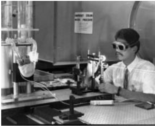
Using laser imaging technology developed for coal slurries, a federal researcher analyzes simulated blood flow through an artificial heart.
