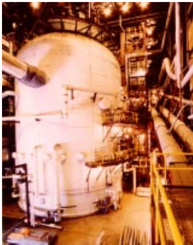
The 70-megawatt Tidd Pressurized Fluidized Bed Combustor pioneered a new, cleaner way to burn coal in utility power plants.
