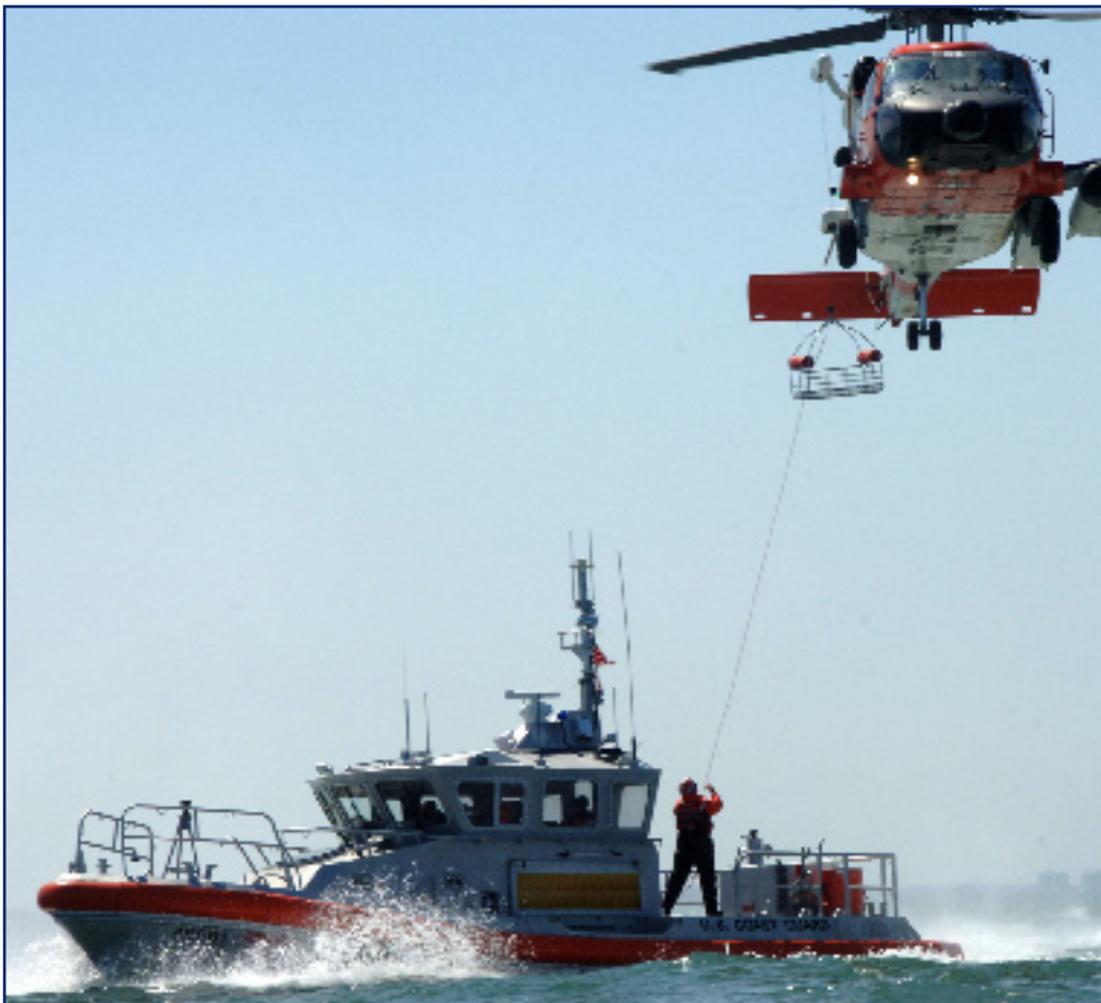
The Coast Guard is modernizing its fleet of 42 HH-60J aircraft with improved avionics, all-glass cockpit displays, new sensors and other mission capability enhancements. The conversion will boost the HH-60T Jayhawks' abilities to interact with and support other new assets, such as the 45-foot Response Boat-Medium. U.S. Coast Guard photo by Petty Officer 2nd Class Christopher Evanson
