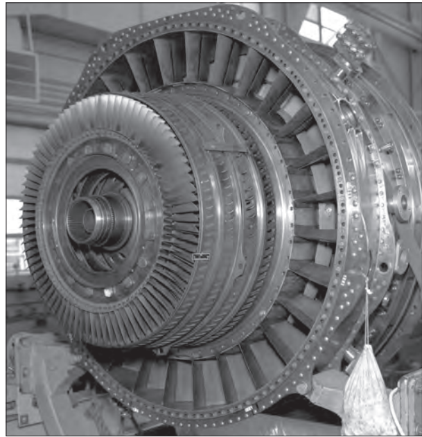
Image 121: A Pratt & Whitney TF30 engine being prepared on 10 August 1967 for a test in PSL No. 1. (NASA C-1967-02809)
