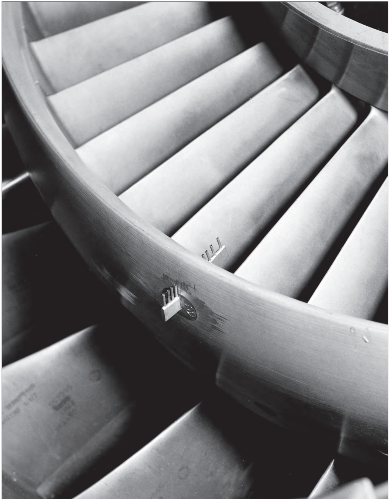
Image 114: A close-up of the Pratt & Whitney TF30 turbofan engine with instrumentation installed on 11 August 1967. (NASA C-1967-02827)
