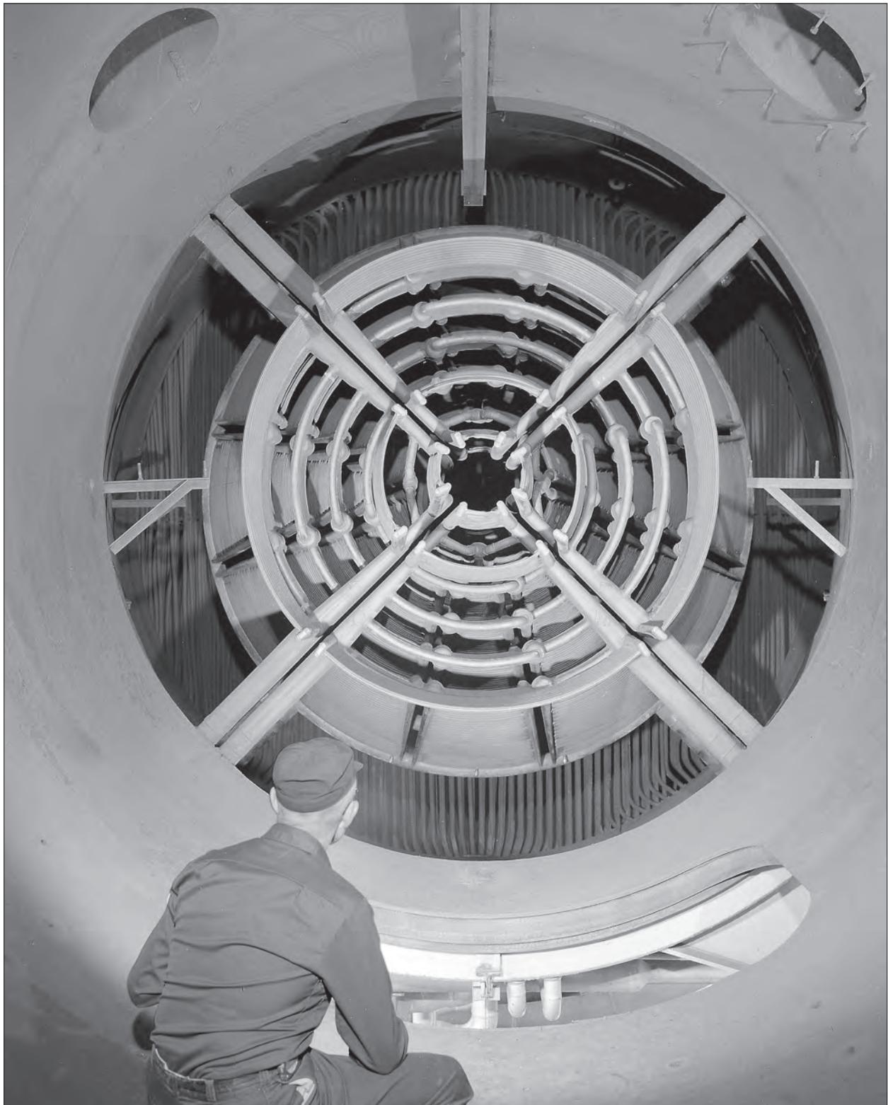
Image 118: Bud Meilander views the flamespreader in PSL No. 2 on 18 May 1967. As the engines being tested in the PSL increased in size, the primary cooler became damaged by the higher temperature exhaust flows. The flamespreader slowed the flow of hot gases at the cooler inlet by spreading the exhaust over a larger area. This increased the cooler's heat-transfer capabilities and prevented damage to the cooler tubing. 10 (NASA C-1967-01733)
