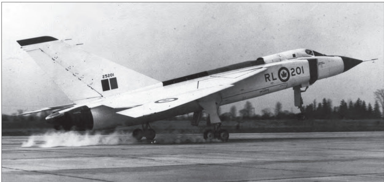
Image 89: Brake testing of the Avro Arrow fighter with substitute engines. The aircraft, without the Iroquois engine, was tested extensively in the mid-1950s, including on missile boosters launched from the NACA Langley Aeronautical Laboratory. (Canadian Department of National Defense)
