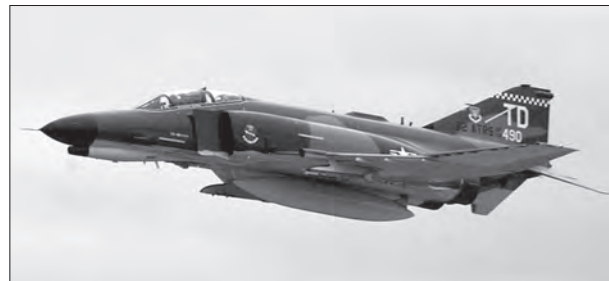
Image 88: F-4 Phantom powered by two J79 turbojets, 2005. (U.S. Air Force)
