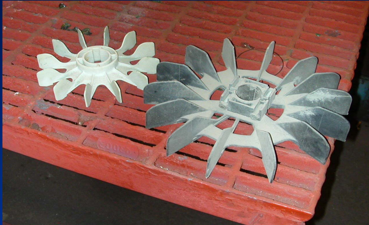
Motor Fan – Premium Efficiency (Left), Standard Efficiency (Right)
