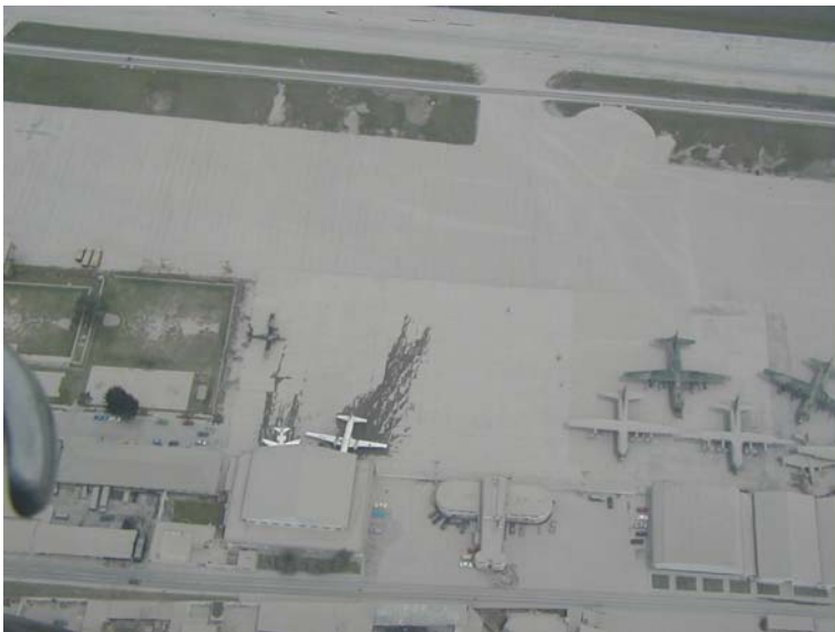
Fig. 2 Photograph taken from the air of volcanic ash from the 3 November 2002 eruption of Reventador covering surfaces at Mariscal Sucre International Airport in Quito. The airport was closed for 8 days as a result of 3–5 mm of ash deposition on planes and runways. Source: Photo by Hugo Yepes, Geophysical Institute of Ecuador
