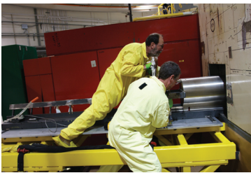
Pee Wee (new cold source for MACS) goes in...it's all connected...and Bob Williams says, Look!...no leaks!
