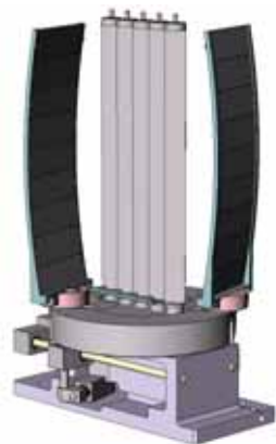
FIGURE 3. CAD image of the double crystal analyzer of which there will be 20 in the MACS detector system.
