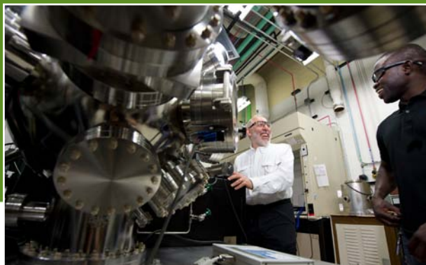
NREL Research Fellow David Ginley (center) and NREL post-doc Paul Ndione operate NREL's new pulsed-laser deposition system, which allows them to deposit multiple graded films on top of one another. This process can create thousands of different compounds on a single 2-inch-by-2-inch substrate.
