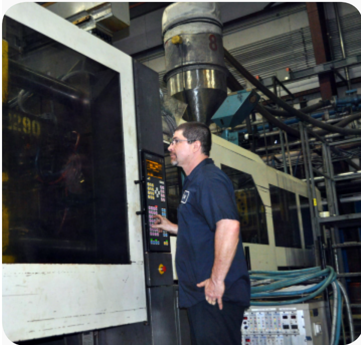
Employee at Accuma Corporation molds plastic into car battery casing.
