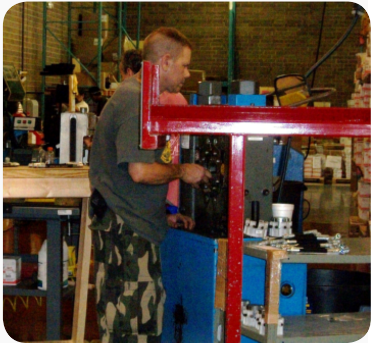
Brian Hobbs completing the hydraulic hose assembly process at DeeTag USA, Inc.
