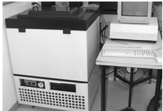
Figure 2. Large Cavity Battery Calorimeter
