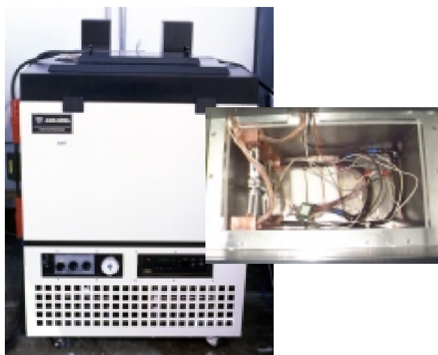
Fig. 1 NREL Heat Conduction Calorimeter (on the left) and its Test Chamber containing Cells (on the right)
