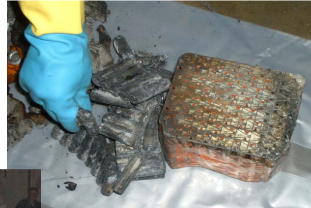
Aftermath of an external short incident
