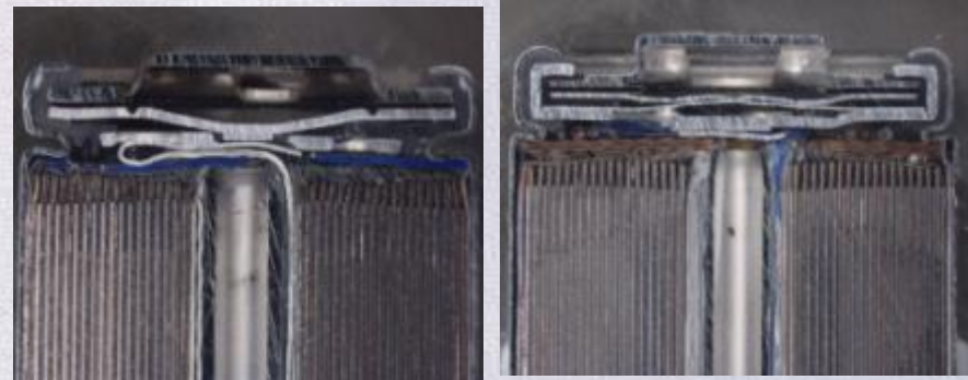
Cross sections of candidate Li-ion cell designs
