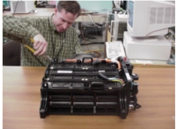
Figure 2 Insight Battery Pack Removed
