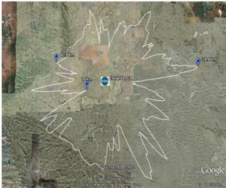
Figure 9. 2.15 dBW Coordination contour around Edwards, CA Telemetry Station
