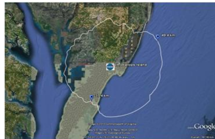
Figure 8. 2.15 dBW Contour around Wallops Island Earth Station
