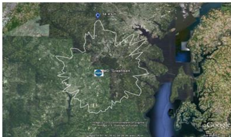
Figure 7. 2.15 dBW Contour around Greenbelt, Md
