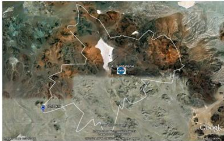
Figure 5. 2.15 dBW Coordination contour around Goldston, CA
