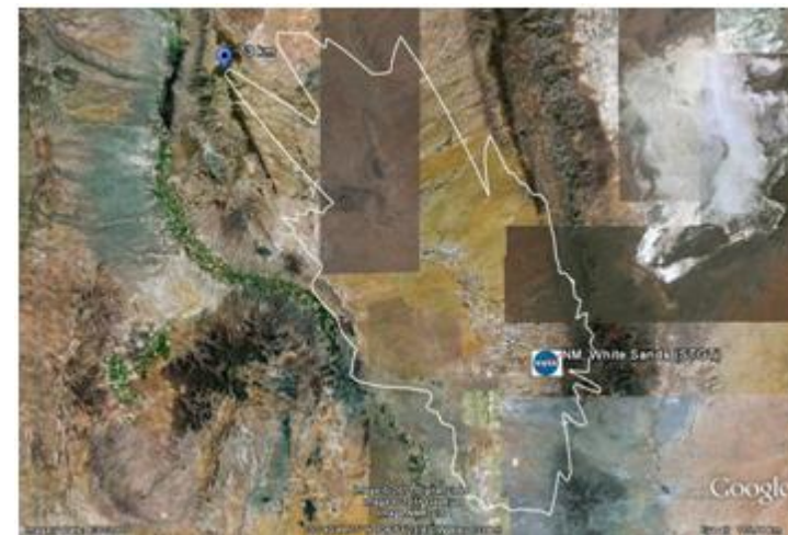
Figure 6. 2.15 dBW Coordination contour around white Sands, NM
