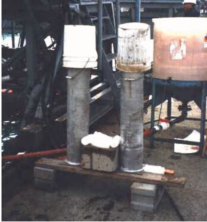
Figure 5. Steel columns used to hold 24-hour water samples (plastic buckets are to prevent rain entering tops)
