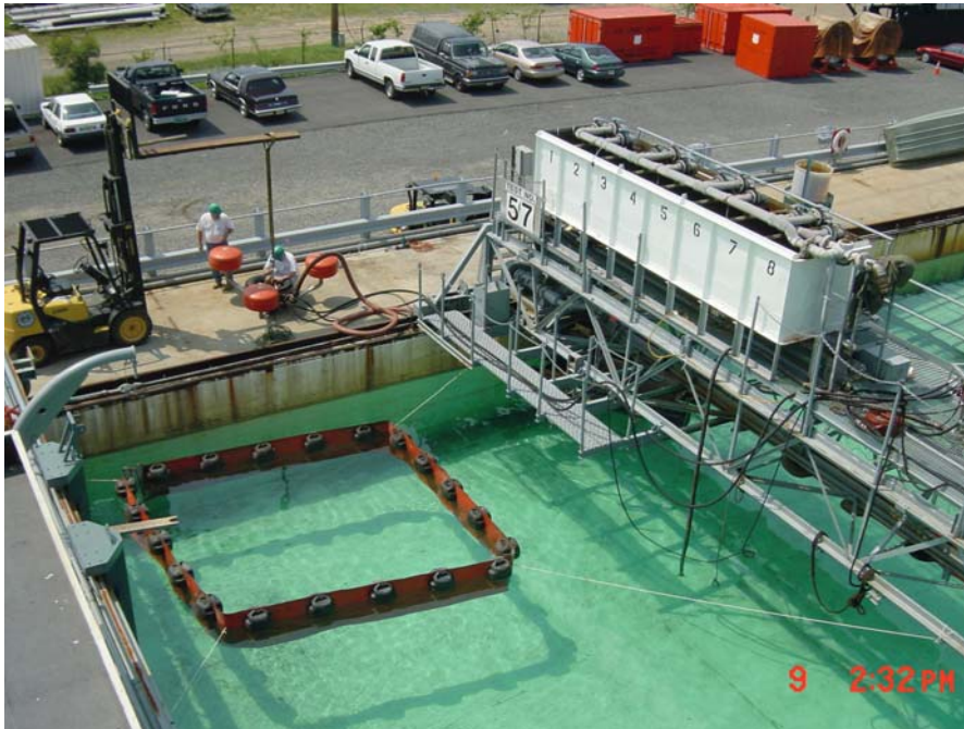
Figure 1. Boomed test area between main and auxiliary bridges.
