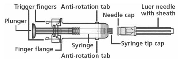
NOTE: Please use the enclosed needle for administration. If a different needle is chosen, it should fit securely on the syringe and be no longer than 1 inch to ensure proper functioning of the needle
