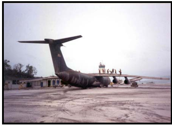
The C-141 on which we had placed couriers on 14 June, damaged on the flightline by volcanic ash.
