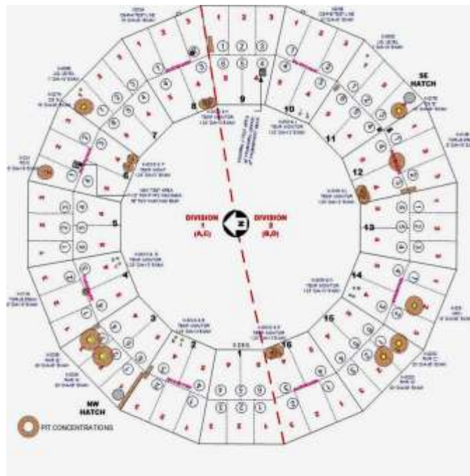
Figure C.1-3 Example of pitting corrosion concentrations in torus
