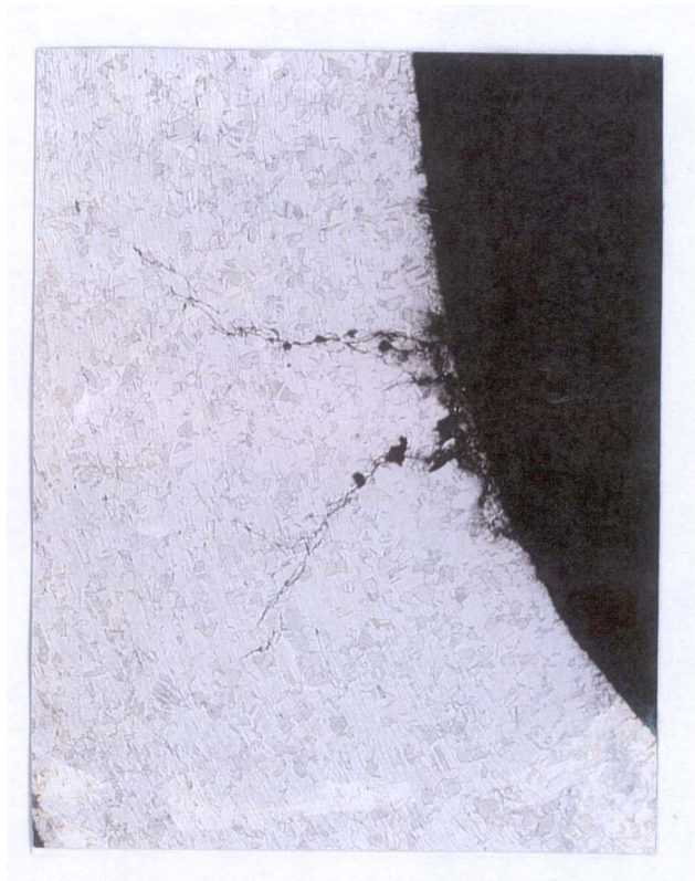
Figure 39 Pit and Stress Corrosion Crack due to Fly Ash Contact with Austenitic Stainless Steel [SRNL photograph].
