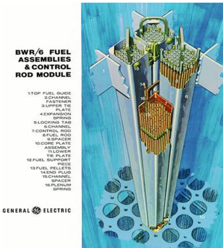
Figure 3 BWR Fuel Assembly [ http://www.nucleartourist.com/images/bwrfuel1.jpg ].
