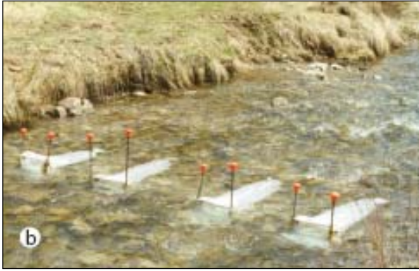
Figure 2. Four bedload traps installed in a relatively small stream, Little Granite Creek, WY.
