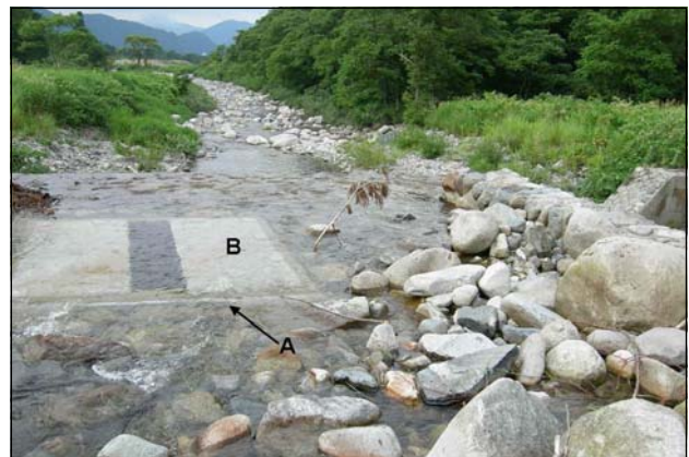
Figure 2. Passive-type acoustic-bedload monitoring in the Uonogawa River, Japan, 2006. A: Pipe geophone; B: Reid-type (formerly referred to as a Birkbeck-type) slot sampler. Downstream view.
