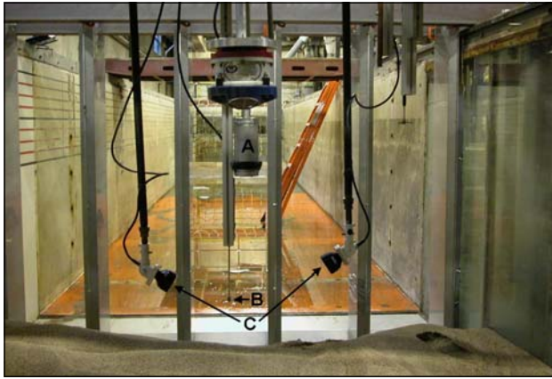
Figure 1. Active-type acoustic-bedload monitoring apparatus over a sand bed in the drained Main Flume, St. Anthony Falls Laboratory, Minneapolis, Minnesota, February, 2006. A: Acoustic-Doppler current profiler; B: Near-field flow-velocity sensor; C: Submersible lights (photo courtesy of Colin Rennie and Rauf Ramooz, University of Ottawa). Downstream view.
