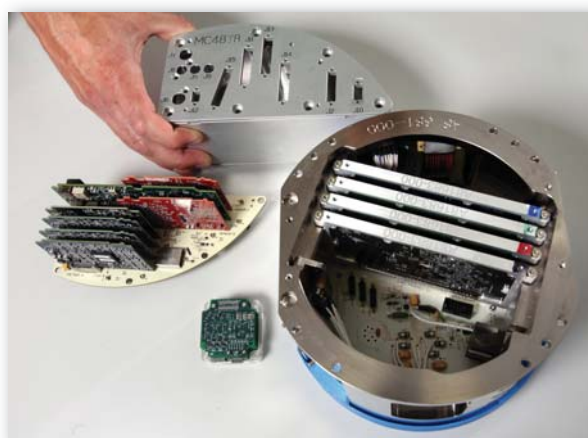
THE DIFFERENT CONFIGURATIONS of the Micro-Modular Telemetry architecture. On the left (the crescent shaped pieces) is the card-based system used in the B61 and in the center and right is the distributed modules architecture used in the W88.
