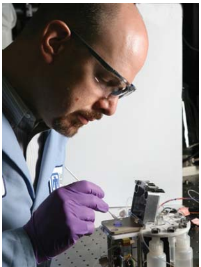
MICHAEL BARTSCH (8125) introduces a buccal swab sample into the Battlefield DNA Analysis extraction module. (Photo by Dino Vournas)
