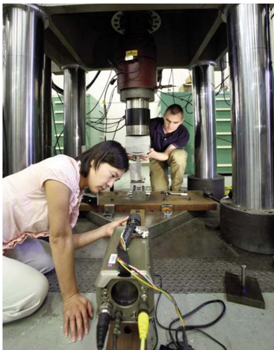
BREAK TIME — Helena Jin and Kevin Nelson (both 8526) inspect the test setup for upcoming experiments to determine the breaking strength of weapon case lugs. (Photo by Dino Vournas)
