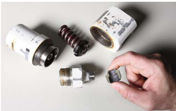
A COMPONENT of this pressure release valve failed, leading to an unintended hydrogen release at an AC Transit fueling station.
