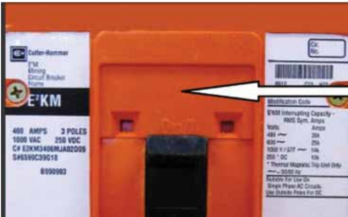
Figure 1 (Note: The arrow in Figure 1 points to an area on the frame of the suspected modified breakers that the MSHA alert notes is smooth. Originally, the E 2 K model had a grey cover and the E 2 KM model a red cover. Also, the breaker's label or frame apparently lacks the mark of a qualified Nationally Recognized Testing Laboratory (NRTL). OSHA knows of no other exterior means of identification.)
