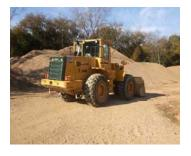
A miner was working underneath a front-end loader with the engine running, checking a hydraulic fluid leak, when the machine moved and rolled over him. The machine was parked on a slight grade, the bucket was raised off the ground, and no wheel chocks were in place.
