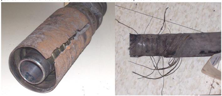
Hammers, punches, and chisels used to force fittings together can cause tiny cracks in the hose ferrule, which over time, may propagate along the entire length of the ferrule, leading to a catastrophic failure of the hose assembly, as shown in the pictures.
