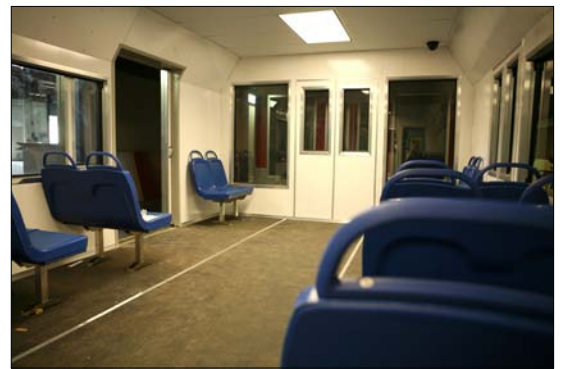
The rail cars are complete with seating and also include sliding doors, lighting, smoke delivery and sound systems.
