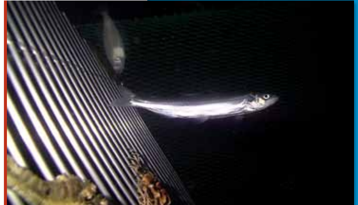
An underwater camera mounted on a bycatch reduction device (BRD) is used to study the escape behavior of eulachon when testing modified BRDs. Here a eulachon is shown being guided upwards and out of a shrimp trawl net by a rigid-grate BRD. Photo: Bob W. Hannah, Oregon Department of Fish and Wildlife, Marine Resources Program.
