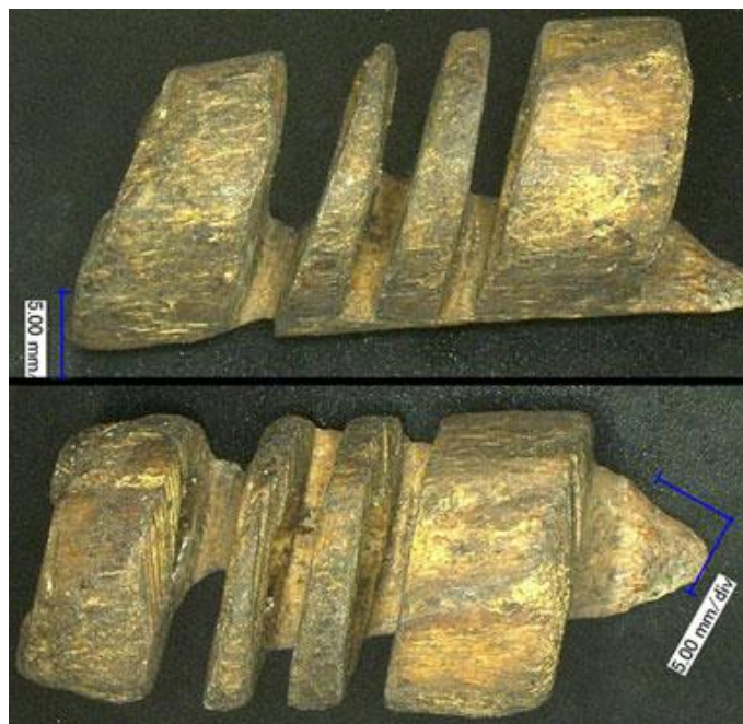
Figure III-25. Two views of numerous identical false starts, which are too uniform for a hand saw.
