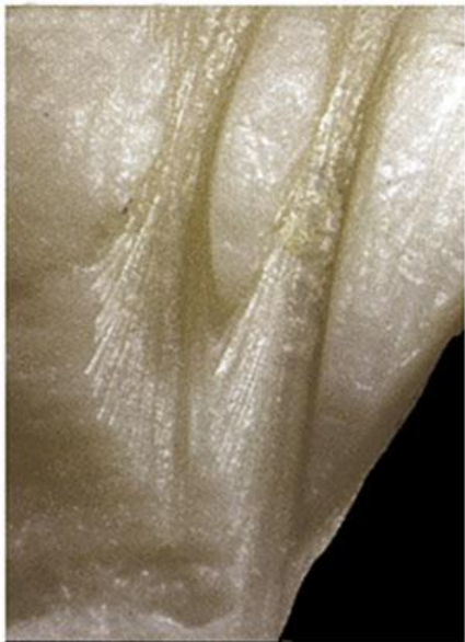
Figure III-35. False start: flare at one end. This suggests the end of the kerf where flexible saw blade is flared due to lateral movement of the handle, while the blade supported by the kerf does not flare.
