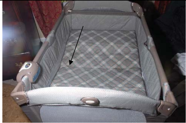
Figure 5b. Incident bassinet play yard – photo from IDI 090213HCC1421 (arrow pointing to v-angle in the mattress pad)
