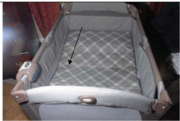
Figure 6. Incident bassinet play yard – photo from in-depth investigation (arrow pointing to V-angle in the mattress pad)
