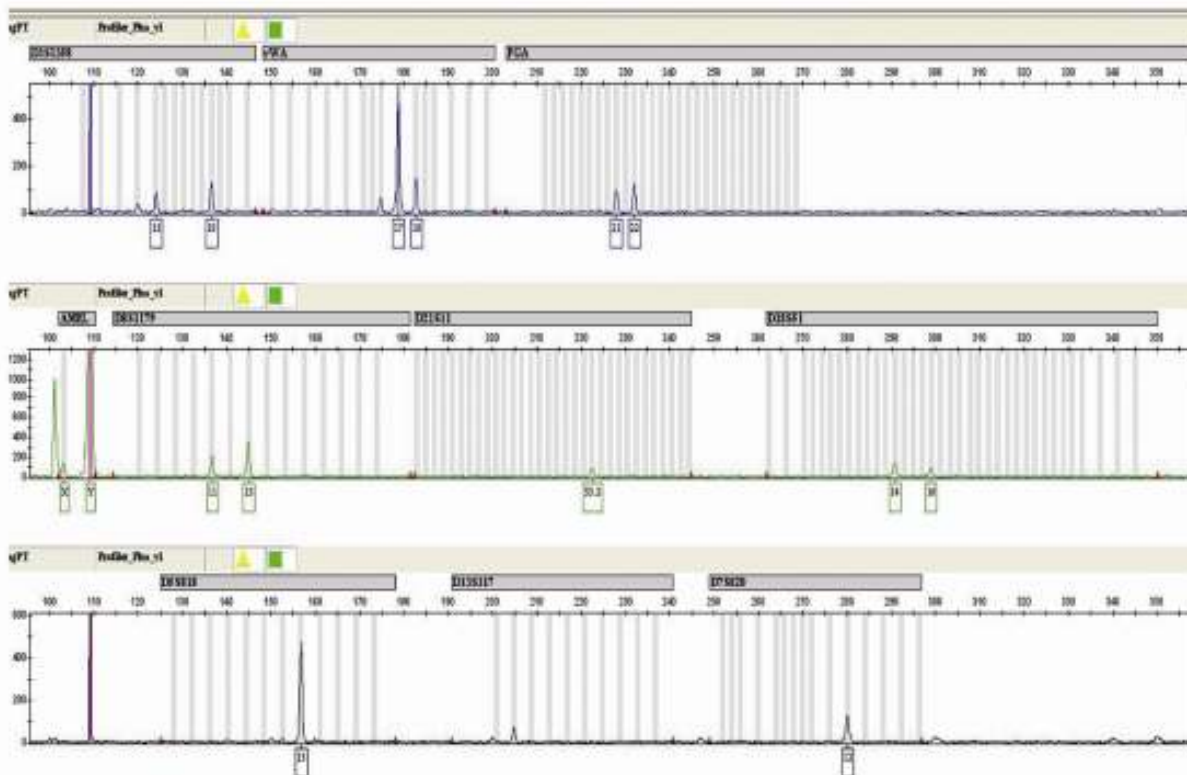
Figure 17: STR electropherogram from dcDOP-PCR amplified sample. Data shown represents all nine STR loci from a single sample (0.03125ng of template DNA amplified). True alleles are marked with a number indicating the STR allele call. For this sample, 13 of 18 of expected STR alleles were detected (72%).
