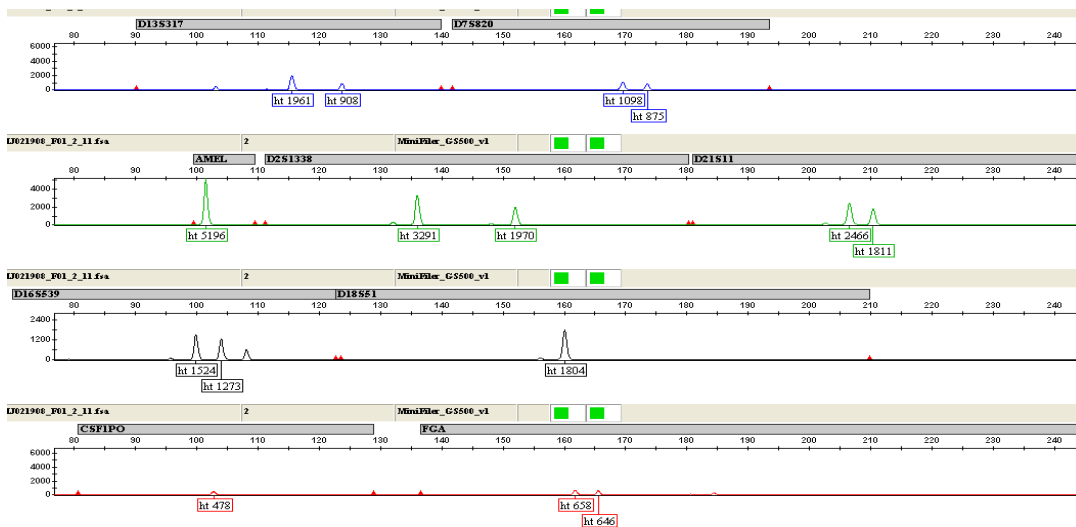
Figure 6: Complete Minifiler™ Profile Generated From 15 White Blood Cells Collected from a Brass Surface and Captured with the PixCell® System
