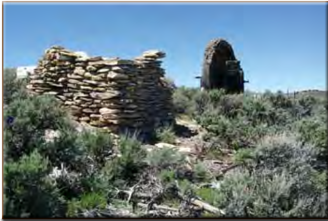
Historic remnants at the Spring Valley Oil Field in Wyoming, which was operational from 1904-1936, show a platform for a steam boiler and a mounted bull wheel
