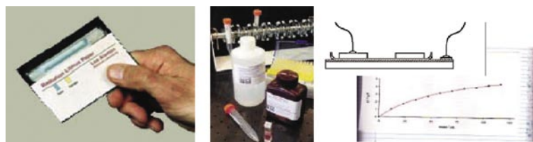
Figures 1-3: Chemical and Radiological Assay Technologies. Radiation Litmus Paper (left) is a low-dose colorimetric radiation dosimeter useful for the military and first responders to a radiological incident. Berylliant (center) is a low-cost beryllium assay, that will reduce the cost of detecting this toxic but indispensable metal. SILM sensors (right) were developed for detecting chemical weapons, and also serve as very low-false positive smoke detectors.
