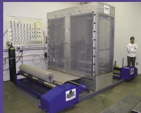
APJeT's textile and plastic coating machine treats a bolt of fabric using the APPJ® technology.
