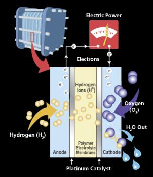
The electrochemical energy conversion in a fuel cell is two to three times more efficient than the internal combustion engine for converting fuel to power.
