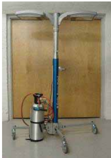
Figure I-4. Pneumatically-telescoping pole completely contracted.
