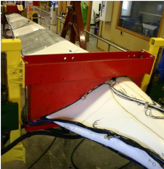
Figure 1. LANL's 9m-Long, CX-100 Wind Turbine Blade Mounted at NREL's Fatigue Test Facility.
