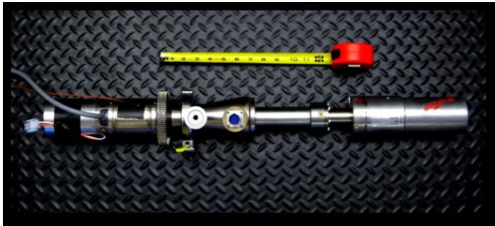
Figure 3. Cryocooler and germanium detector mechanical assembly.
