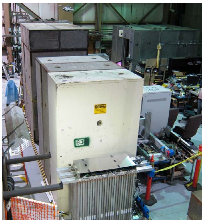
Figure 3. Photograph of the experiment, looking East. Concrete blocks are prominently shown, and the lower MMT detector is in the foreground. The upper detector set is behind the higher concrete stack and not visible.
