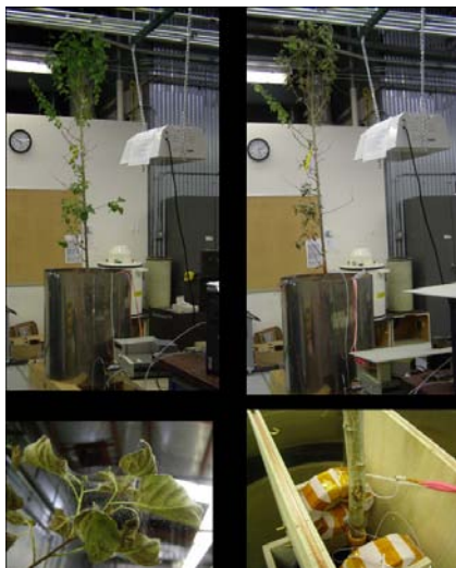
Figure 2. Top Row: Two photos of the tree in the ULF NMR system. The NMR system is located inside the silver magnetic shield. The photo at left was taken ~ 7 days before the photo at right, and significant decline in leaves is noted. Bottom Row: Left shows close up of leaves infected with parasite. Right shows close up of NMR system around tree trunk.
