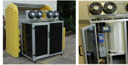
Figure 2. Thermal Storage Unit in a fully instrumented test module that demonstrates on a “bench-scale” the ability to utilize ambient air as a heat sink to reversibly capture and release thermal energy. Preliminary engineering analysis shows that the Thermal Storage Unit operates at a SEER rating of greater than 40.
