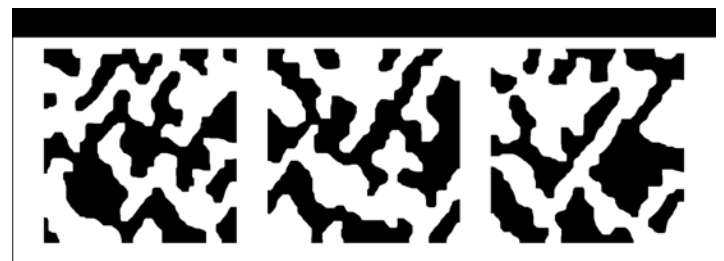
Figure 4. Example of microstructure generation model. The left image served as a target while the center and right images are example of structures that could have come from the same stochastic microstructure process as the target.
