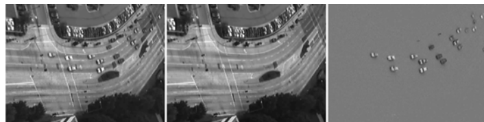
Figure 1. Left: one frame from a video sequence. Middle: corresponding frame from the low-rank component; all moving objects are absent, and road lines obscured by cars in the original frame have been filled in. Parked cars remain; an approach that simply identifies cars would be less useful. Right: the sparse component contains only the moving objects, including a cyclist and pedestrian on the sidewalk. The pedestrian is very difficult to notice in the original video, but is clear in the video sequence of the sparse component.
