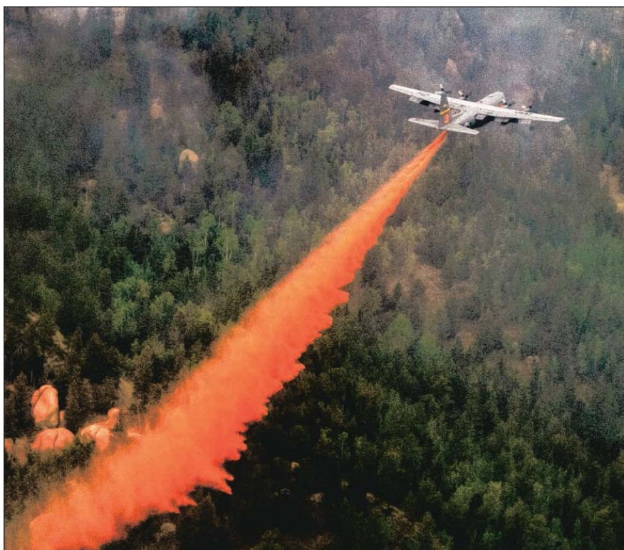
STAFF SGT. STEPHANY D. RICHARDS The 153rd Airlift Wing from Cheyenne WY use a modular air fire fighting system equipped C-130 Hercules aircraft in support of the Waldo Canyon wild fire June 27.
