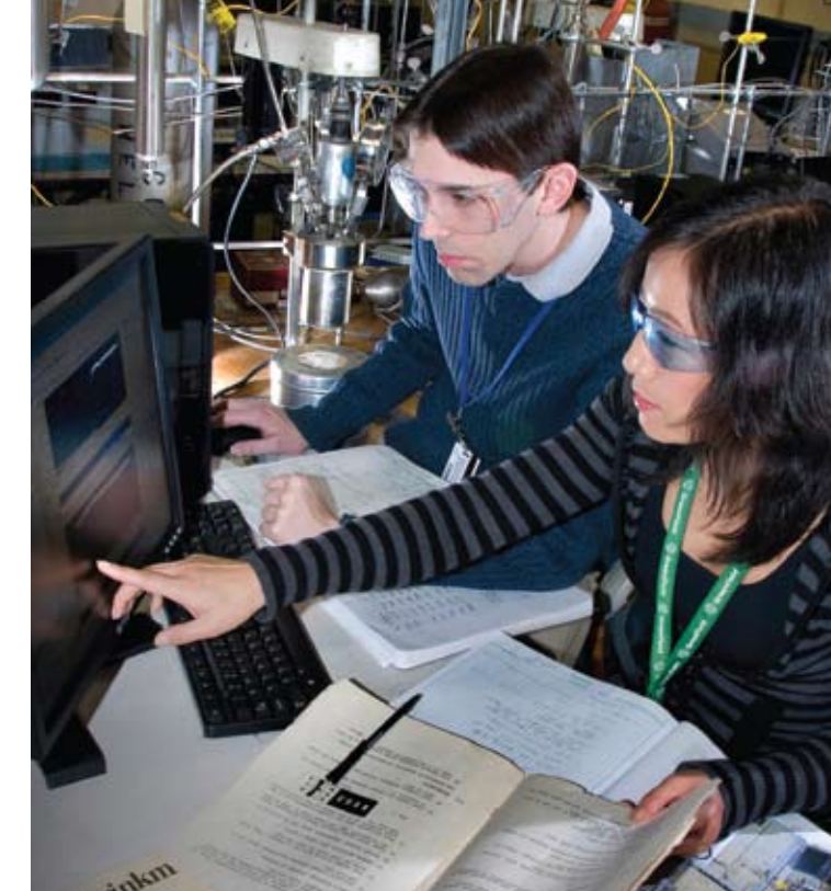
David Lacina and Weimin Zhou prepare a LabVIEW program to measure the hydrogen uptake and release from a complex hydride in solution.
