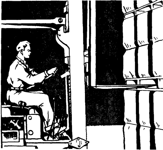
Figure 4-116. Approaching a pallet. Forks must enter at an equal distance from the center stringers.
