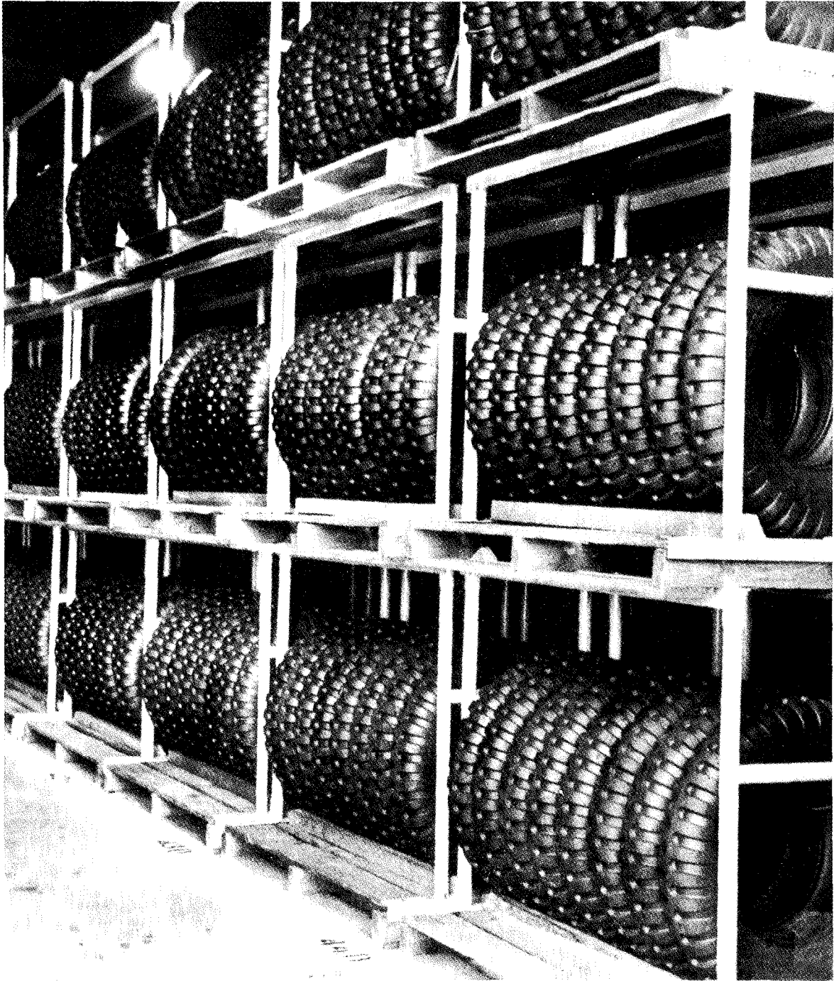
Figure 5-43 Typical storage in pallet support sets
