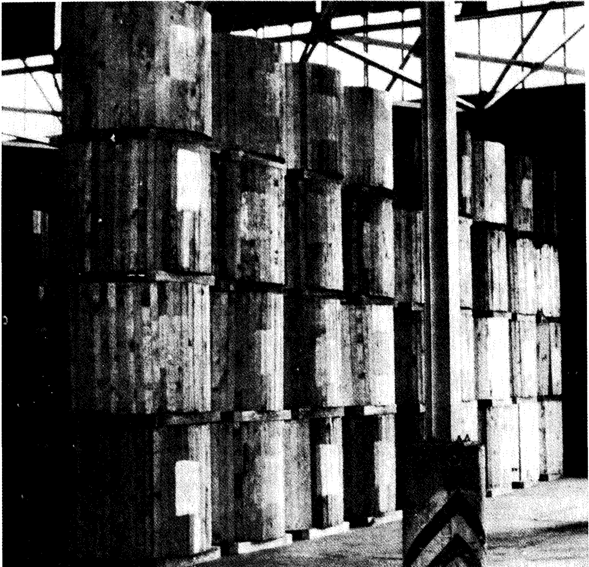
Figure 5-71 Small cable reels properly dunnaged for safe efficient stacking
