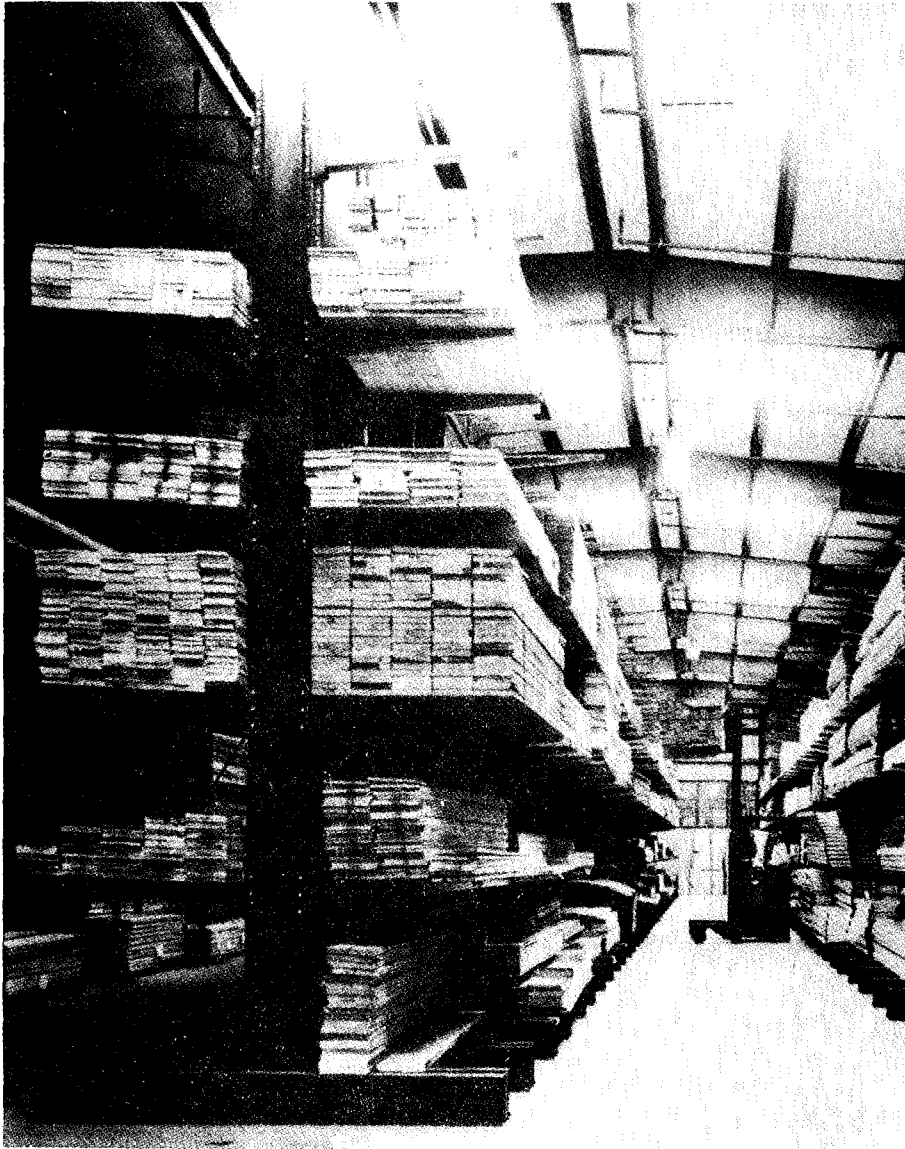
Figure 4-93. Cantilever rack (double face)
