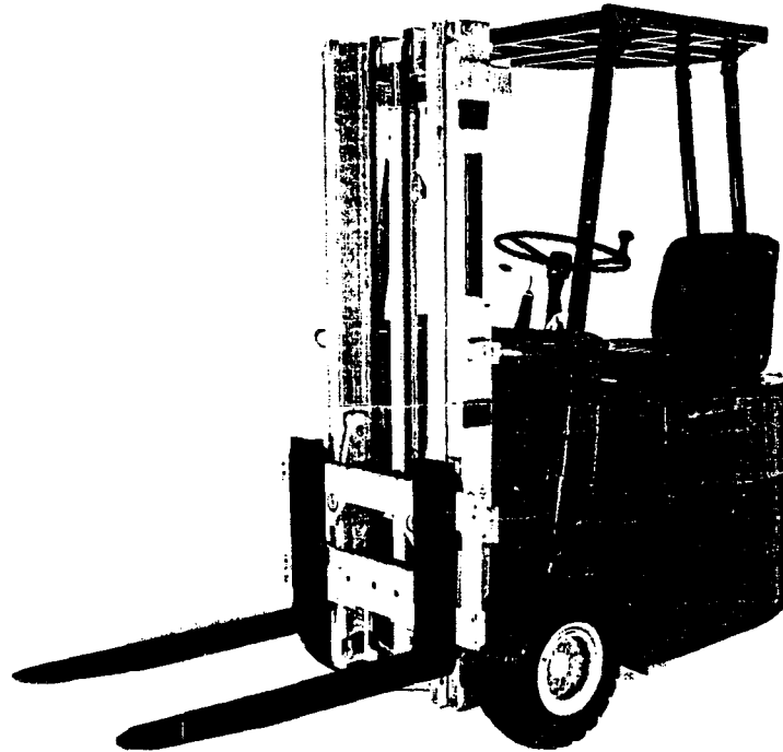
Figure 4-17. Truck, forklift (3-wheel) pneumatic tires, 3,200 pound, 144-inch lift
