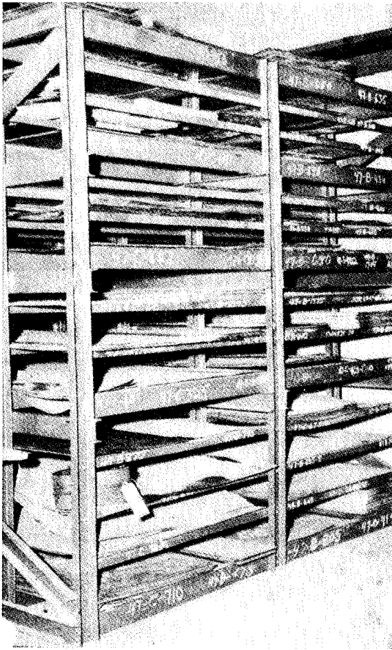
Figure 5-51 Lightweight sheet or strip racks
