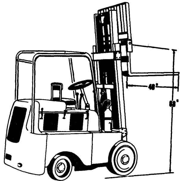
Figure 4-18. Truck, forklift, solid or semisolid rubber tires, 6,000-pound, 127- to 180-inch lift.
