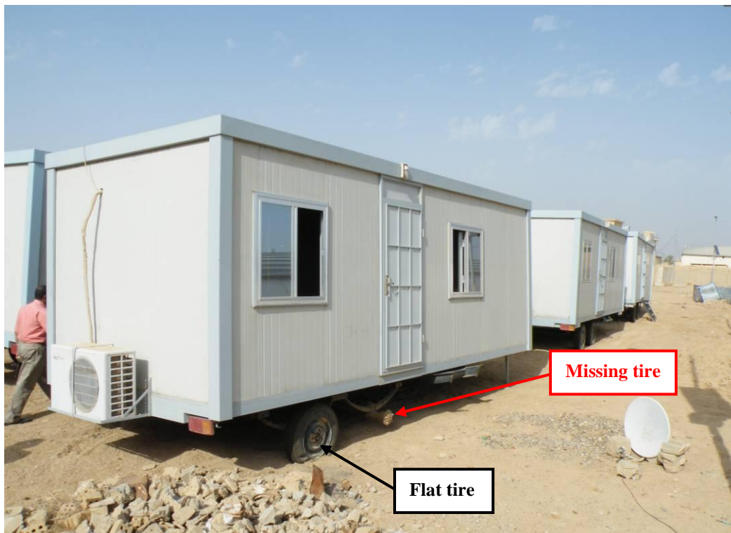
Site Photo 8. Exterior condition of trailers at the MOE’s Ramadi outdoor warehouse facility
