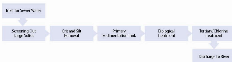
WWTP MULTI-STAGE TREATMENT PROCESS
