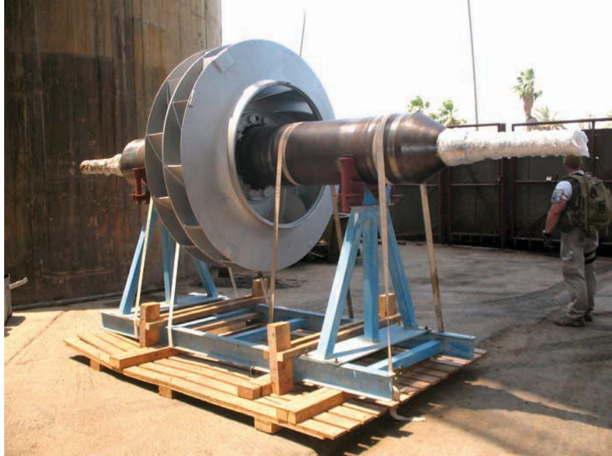
Rebuilt shaft for Unit 6 generator impeller.
